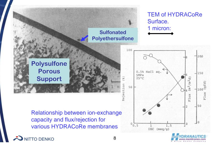
Barrier Layer Cross-Section and Charge Density
